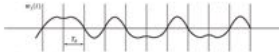
(b) Filtered Polar NRZ Input Waveform
