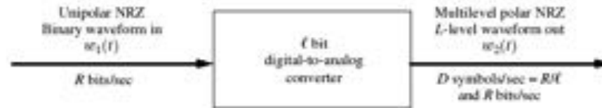
(a) C Bit Digital-to-Analog Converter
